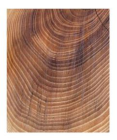
Robinia is indispensable, especially when it comes to topics such as 'use of wood in outdoor areas/installation into the ground' or 'pest-resistant timber'. It is characterised by specific properties such as a high degree of hardness, a low proportion of sapwood and excellent durability. The following table illustrates this and shows how robinia compares to other types of wood:
